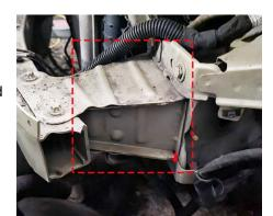
up inside the leg. The maximum size bolt fixing is M16, with a maximum of two permitted in each chassis leg to hold the plate.
